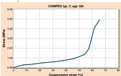
developing a compressible mortar, on which Rotter had already spent considerable time and money. In the 1990’s he was successful in finding two industrial partners to join him. One was a cement manufacturer, the other a polystyrene technology company. A series of lab tests and large scale mixing and pumping tests were performed and the result was a near perfect material named COMPLEX-mortar, which suited all requirements<sup>[9]</sup>.
