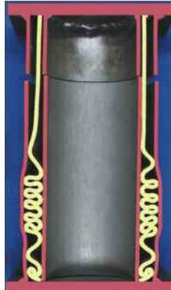
Above, left: Fig 4 – Load displacement diagram for a project designed group of 4 LSC (B. Moritz 2008); Above, right: Section through a yielding element<sup>[7]</sup>
