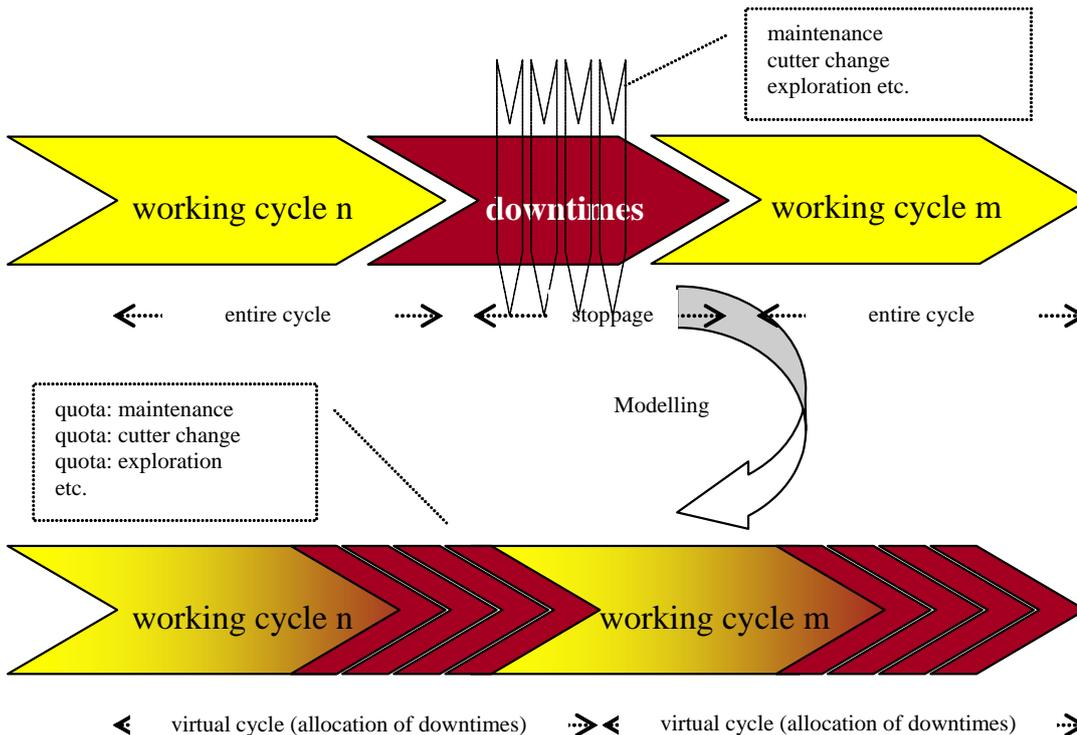
Fig. 1 Allocation of downtimes on the working cycles
