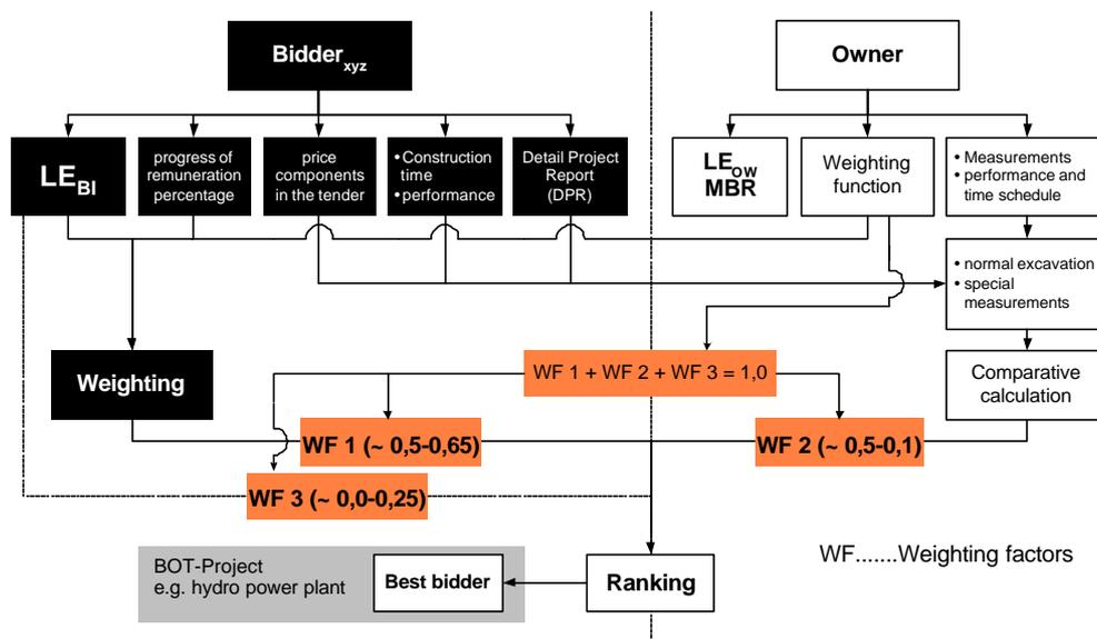
Figure 4. Diagram for determining the best bidder with weighting of relevant tender components.
